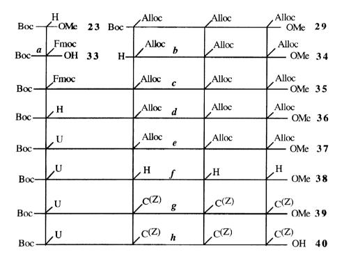
Reagents and conditions: (a) i. NaOH (1N), dioxane; ii. Fmoc-Cl, then HCl (1N) (b) TFA/CH<sub>2</sub>Cl<sub>2</sub> (b) TFA, CH<sub>2</sub>Cl<sub>2</sub> (c) i. 33, CH<sub>2</sub>Cl<sub>2</sub>, DCC/HOSu, 12h ii. 34, NMM (d) CH<sub>2</sub>Cl<sub>2</sub>, DEA (e) 4d, Brop, TEA, DMF, 0°C (f) Pd[P(Ph)<sub>3</sub>]<sub>4</sub>, DEA, CH<sub>2</sub>Cl<sub>2</sub> (g) 4c, TEA, Brop, CH<sub>2</sub>Cl<sub>2</sub>, 0°C (h) LiOH (1N), dioxane, 0°C.
